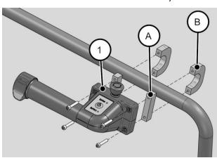
➤ To comply with the specifications as per the IPX4 protection class, observe the horizontal installation position shown below.
